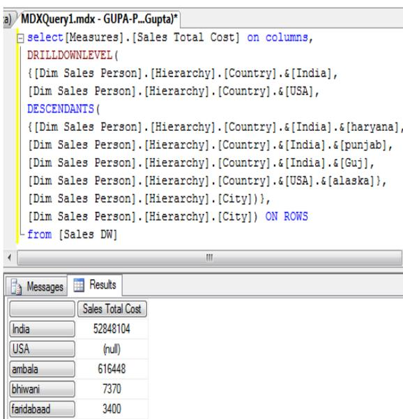
Figure2: Drill-down operation.
