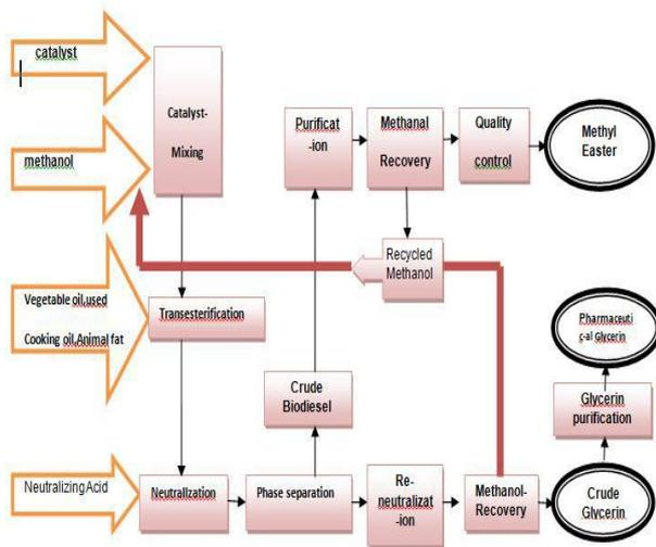
Fig 1. Process of Production of biodiesel
