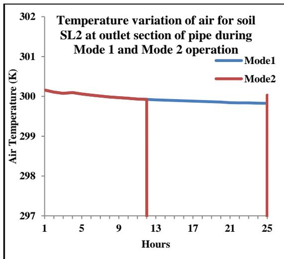
**Figure 5. Hourly temperature of air for soil SL2 at outlet section of pipe (0.1 m diameter) at 5 m/s flow velocity for Mode 1 and Mode 2**
