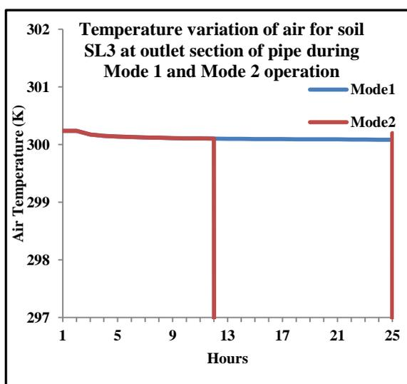
**Figure 6. Temperature of air for soil SL3 along the length of pipe (0.1 m diameter) at 5 m/s flow velocity for Mode 1 and Mode 2**
