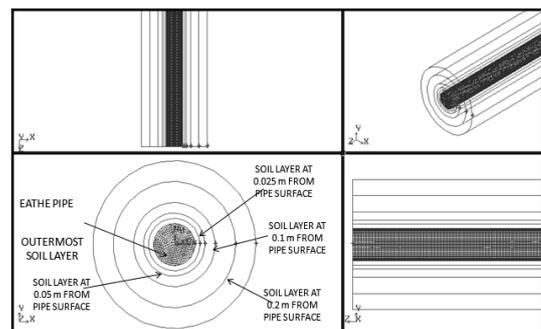
Figure 1. Four different views of CFD model for EATHE
