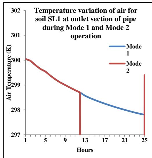
Figure 4. Hourly temperature of air for soil SL1 at outlet section of pipe (0.1 m diameter) at 5 m/s flow velocity for Mode 1 and Mode 2
