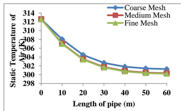
**Figure 3. Validation of EATHE system**
