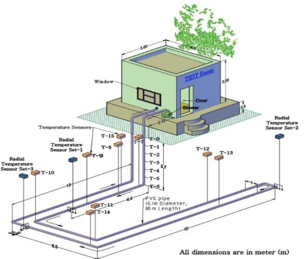
**Figure 2. Schematic of room integrated EATHE system**
