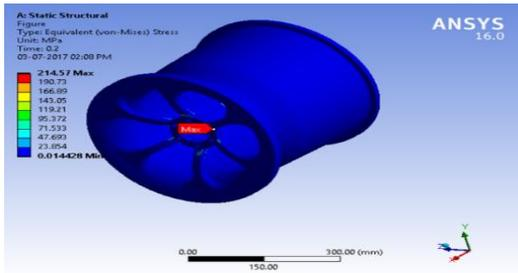
Fig- 6: Stress levels in alloy wheel
