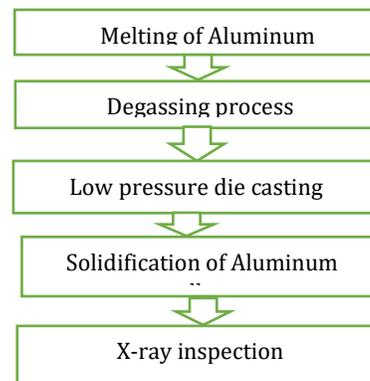
**Fig1:** Steps of Alloy Wheel Production Process
