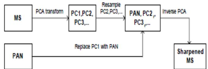
Figure 1 Flow diagrams of the PCS sharpening
