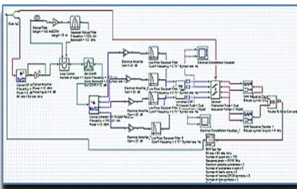
Fig -3: Block Diagram of 112 Gbps DP 16-QAM Coherent receiver.
