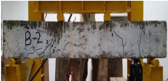
Fig 12:- cracked pattern of beam
