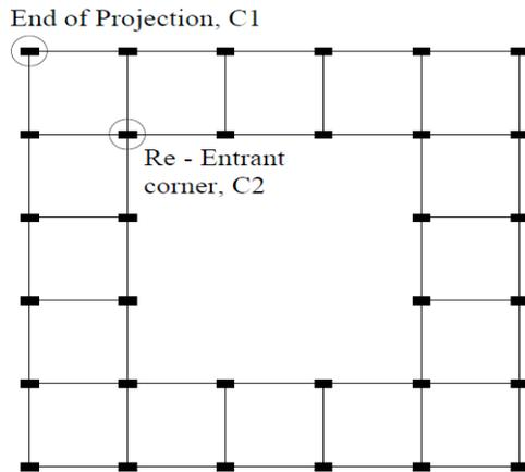
Fig-4: Beam and column layout of model.
