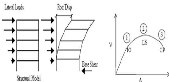
Fig-3: Building model and pushover curve.
