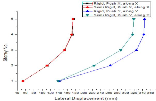
Chart-1: Variation of lateral displacement- mass regular, at the re-entrant corner and at the end of the projection
