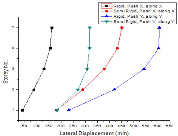
**Chart-12:** Variation of lateral displacement – mass & stiffness irregular (at the re-entrant of corner and at the end of projection)
