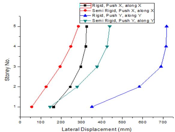
Chart-2: Variation of lateral displacement- mass irregular, at the re-entrant corner and at the end of the projection
