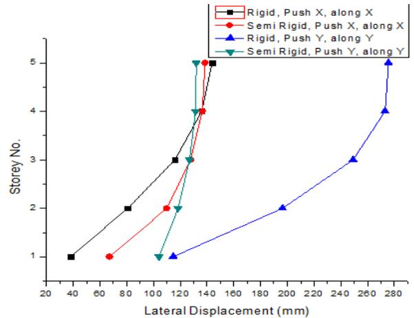
**Chart-11:** Variation of lateral displacement – mass & stiffness regular (at the re-entrant of corner and at the end of projection)
