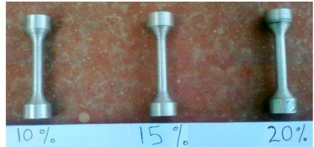
Fig(2): Tensile Strength Specimens of different composition
