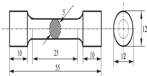
Fig (1) :The dimension of standard specimen for tensile test.
