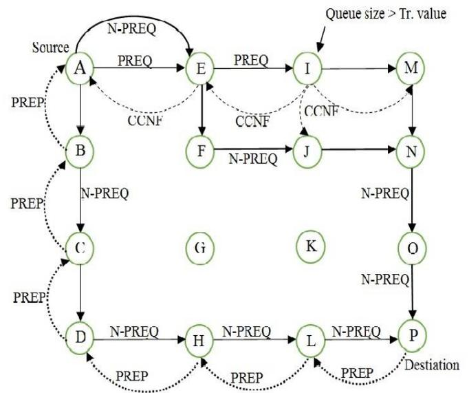
Fig -1: Modified PREQ in HWMP
