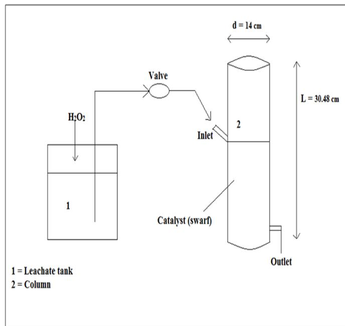
Fig 2.1: Schematic flow diagram of experimental set-up of the Fenton reactor
