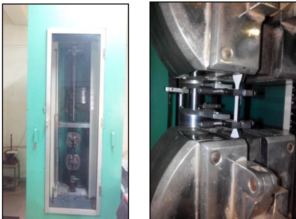
a. UTM Machine b. Extensometer Position
