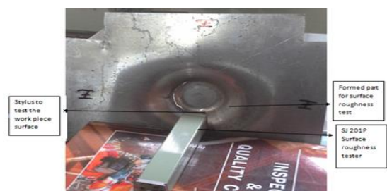
Fig 10: SJ-201P surface roughness testing of formed part
