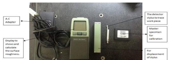
Fig -9 Mitutoyo SurfTest SJ-201P (Surface Roughness Tester)
