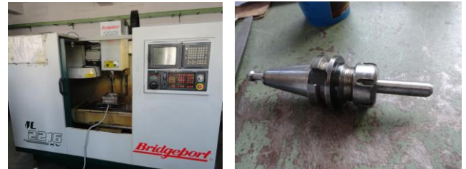
Fig -4(a): Overview of CNC milling machine (VMC) and Fig -4(b): Stainless steel tool of diameter 20 mm
