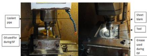
Fig -7: Lubrication system used during ISF
