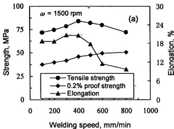
Figure 5 Effect of welding speed on mechanical properties
