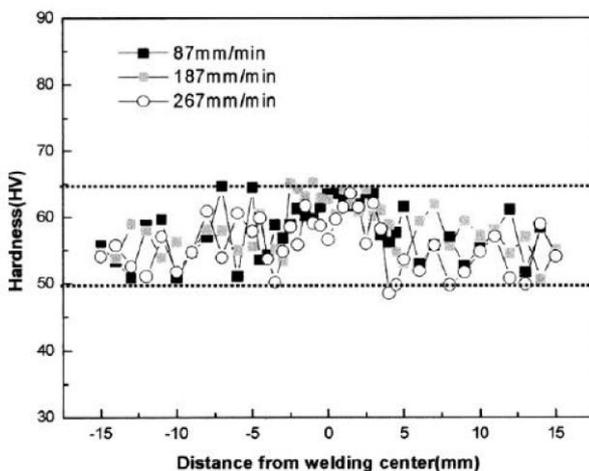
**Figure 6.** Effect of welding speed on micro-hardness
