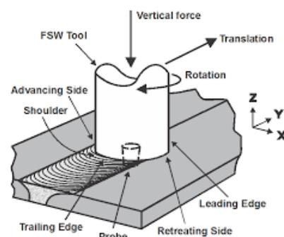
Figure 1: Mechanism of Friction Stir Welding
