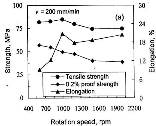
Figure 4. Effect of rotational speed on tensile properties [8]
