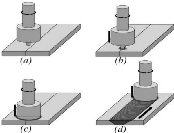
**Figure 2:** FSW Working Processes: (a) Starting position, (b). Start of joining, (c). Insert joining tool and (d). Joining [3,5]
