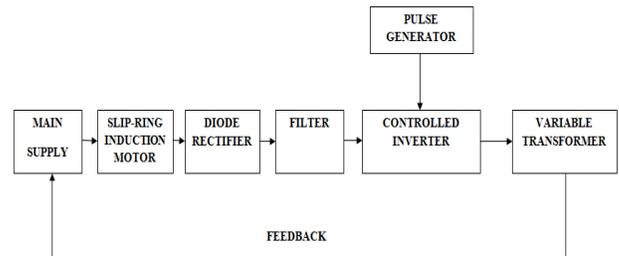
Figure 2 Block Diagram of Slip Power Recovery Scheme with Variable Transformer Turn Ratio
