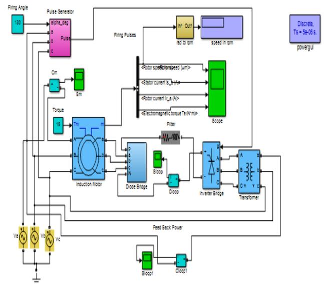
Figure 3 Simulation Model of SPR Scheme with Turn's Ratio Control
