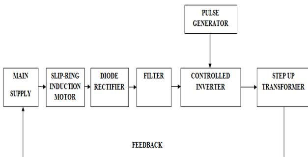
Figure 1 Block Diagram of Conventional Slip Power Recovery Scheme
