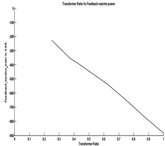
**Figure 4(c) Graph between T-Ratio and Feedback Reactive Power**
