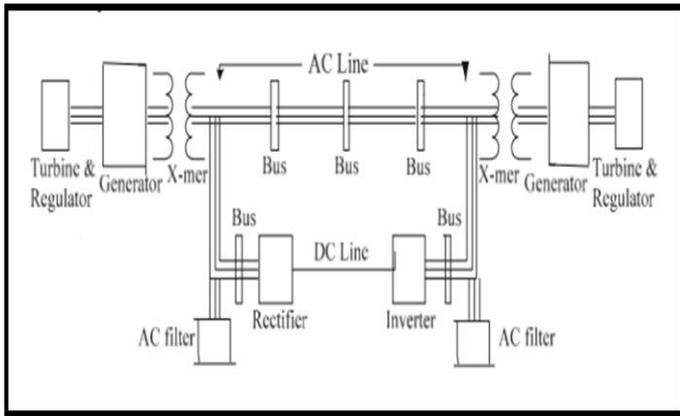
Fig. 3. Block diagram of proposed transmission network
