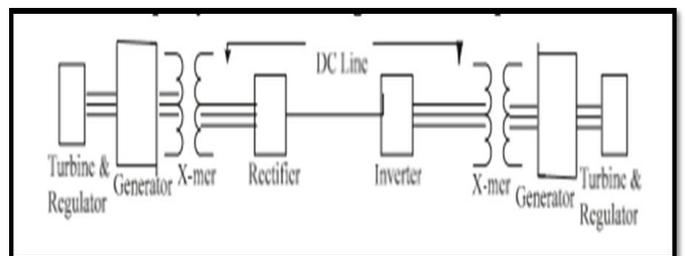
Fig. 2. Basic Scheme for composite AC-DC Transmission
