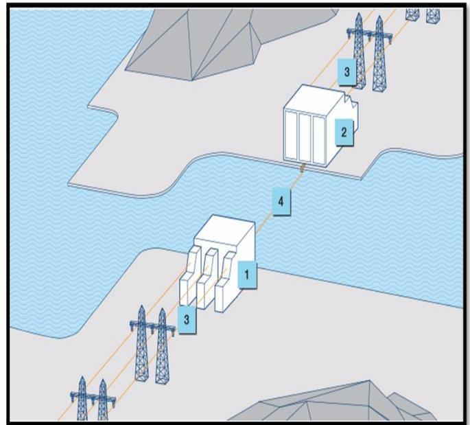
Fig 1- 1 HVDC converter station rectifier | 2 HVDC converter station inverter | 3 Alternating current (AC) | 4 Direct current (DC)
