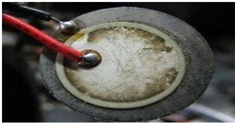
Figure 3.2 Metal disk with piezoelectric disk attached, used in a buzzer.
