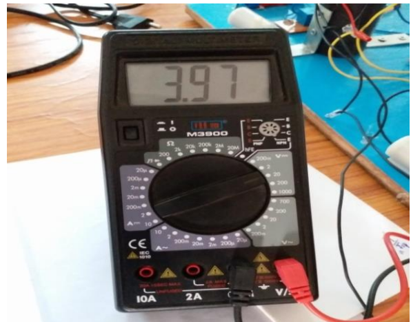
Fig.5.4 Output from Piezo Electric Panel
