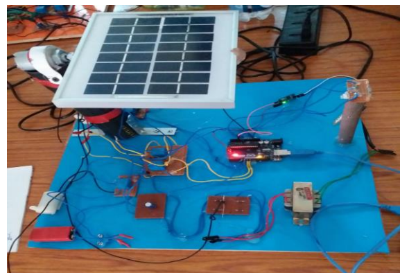
Fig.5.1.Implemented hardware with solar panel at top
