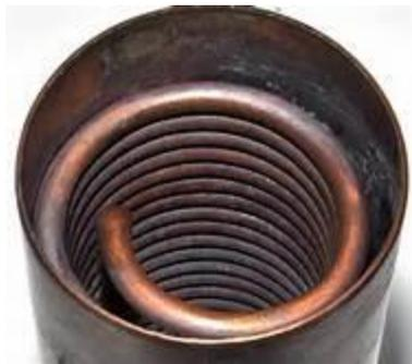
**Fig-3:** Copper tube coiled condenser
