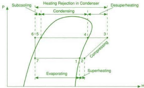
Fig. 2: P-h diagram with sub-cooling and super heating [4]
