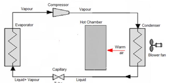
Fig. 7: Compression Refrigerator Systematic Diagram [6]
