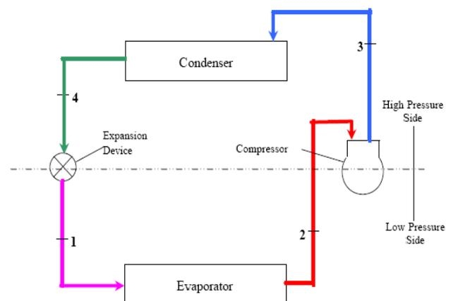
Fig. 1: vapour compression refrigeration cycle [4]
