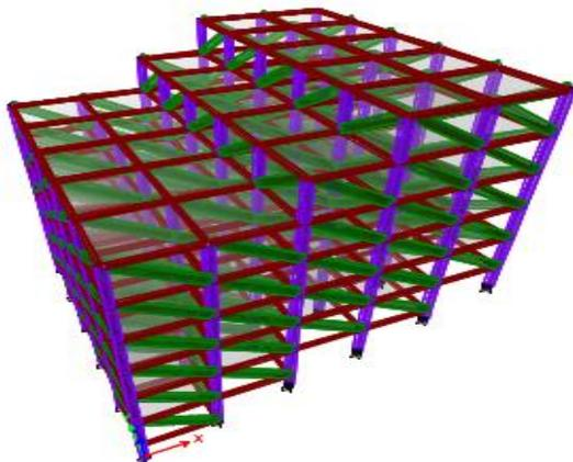
Fig 2.3 : Building with sloping angle 20°
