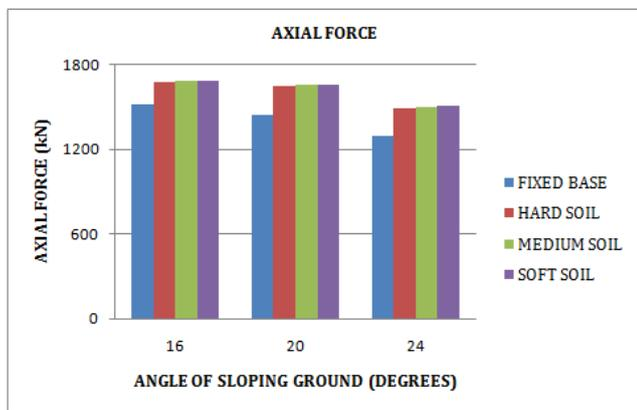
Fig 3.4 Axial force for building on sloping ground with and without soil structure interaction
