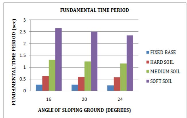
Fig 3.3 Fundamental time period for building on sloping ground with and without soil structure interaction.
