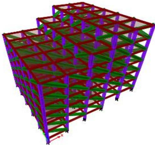
Fig 2.2 : Building with sloping angle 16°
