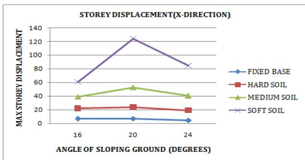
Fig 3.2.1 Maximum storey displacement for building on sloping ground with and without soil structure interaction in x-direction.
