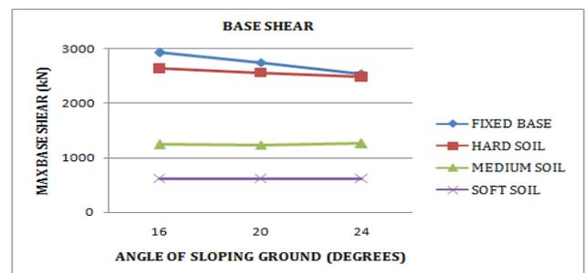
Fig. 3.1 Base shear of the building on sloping ground with and without soil structure interaction
