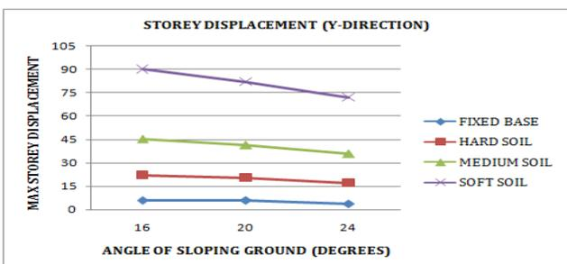
Fig 3.2.2 Maximum storey displacement for building on sloping ground with and without soil structure interaction in y-direction.
