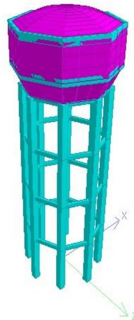
Fig 3 Framed Type model prepared in Staad-Pro
