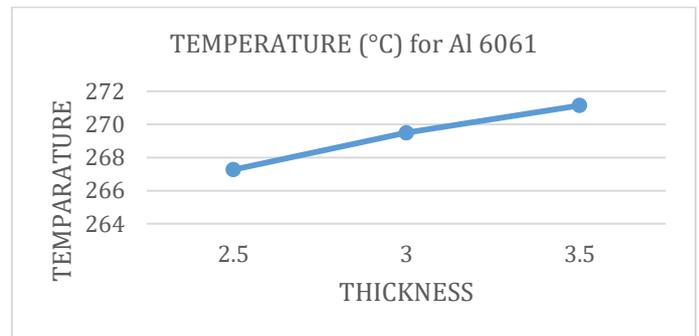
**Fig-8:** Graphical representation of temperature Distribution results with ANSYS for Rectangular Fins of Aluminium Alloy 6061 with variable size fin thickness.
