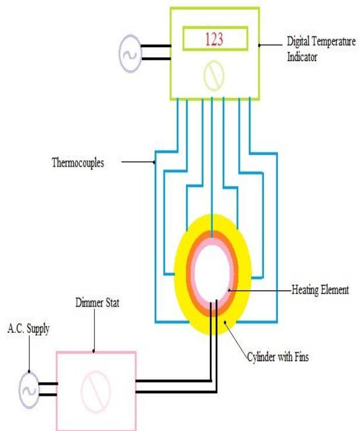
**Fig-4:** Experimental setup for measurement of temperature at tip of the fin.
