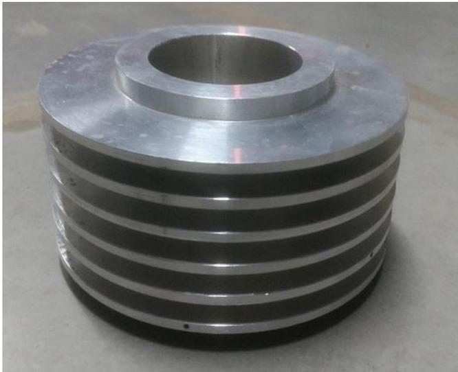
**Fig-3:** Cylinder with 3.0 mm thick rectangular fin.
