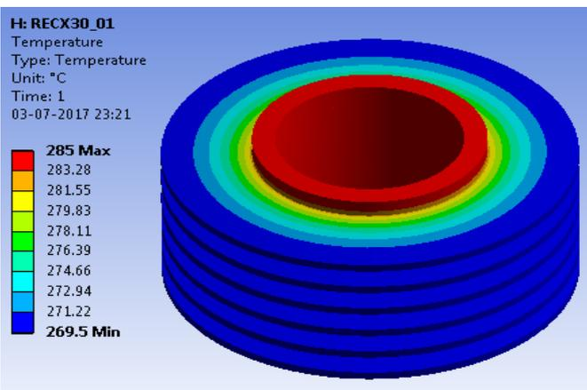
**Fig-7:** Temperature Distribution for Rectangular Fins of Aluminium Alloy 6061 with 3.0 mm Fin Thickness
