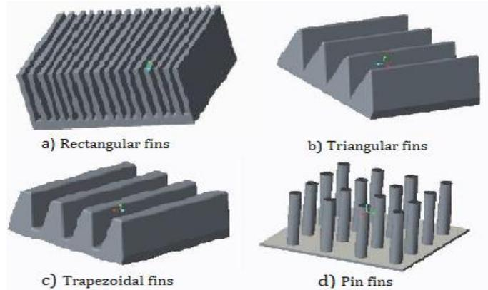
Fig-1: Different types of fin geometries
