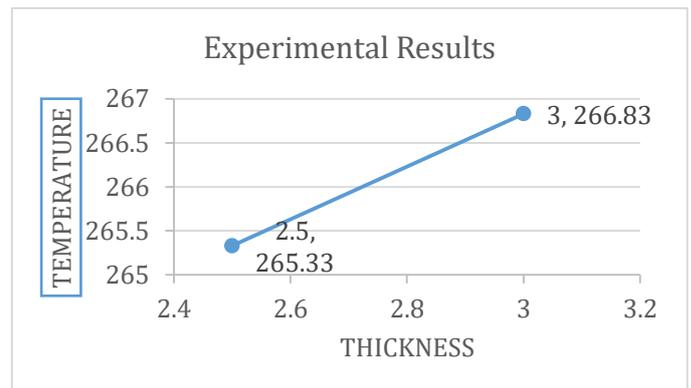
**Fig-9:** Graphical representation of temperature Distribution results with Experimental Model for Rectangular Fins of Aluminium Alloy 6061 with variable size fin thickness.
