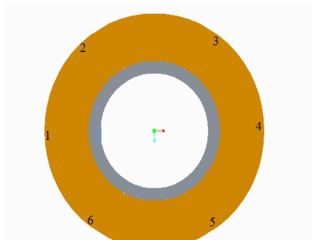
**Fig-3:** Placement of thermocouples.
