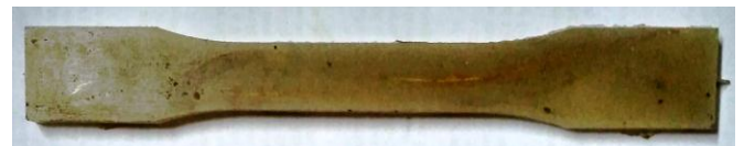
Fig-13 Epoxy + Coconut Fiber Test Specimen
