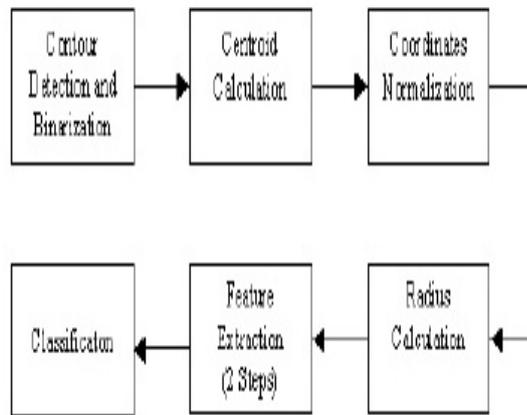
Above block diagram describes the process for ear detection.
