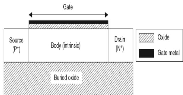
Fig-3: Schematic of a p-channel p-i-n TFET [12]
