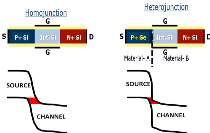
**Fig-9:** Tunneling Current with Homo and Hetro-junction
