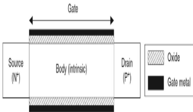
Fig-4: Schematic of p-channel Double Gate TFET [19]
