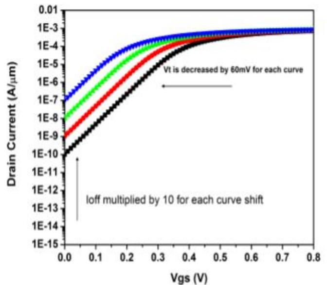
Fig-2: MOSFET Transfer characteristics with reduction in  $V_T$  [5]
