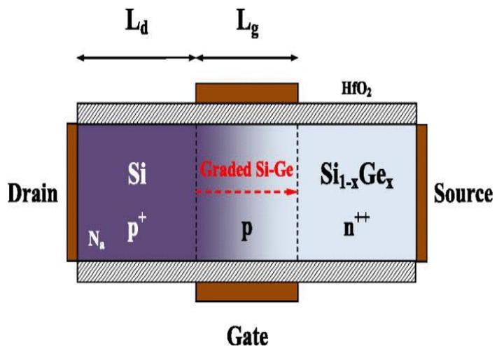
Fig-8: Structure of Hetero-junction TFET [21]
