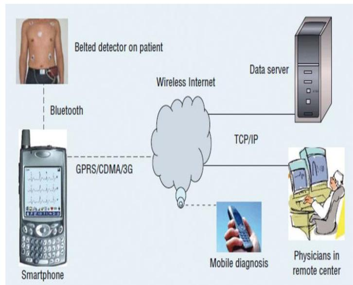
Fig -2: A typical remote diagnosis model
