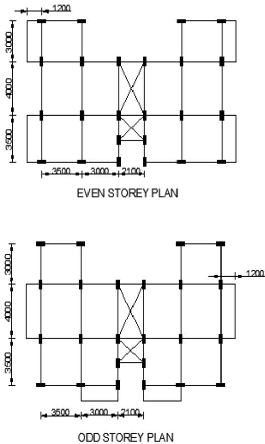
Fig1: Plan of building G+7
