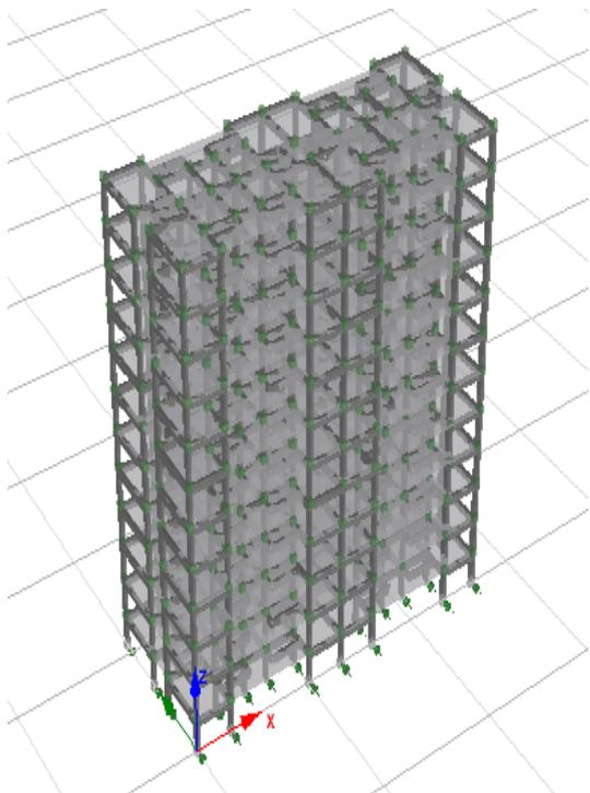
Fig 6: SeismoStruct Model of the building of G+11 building
