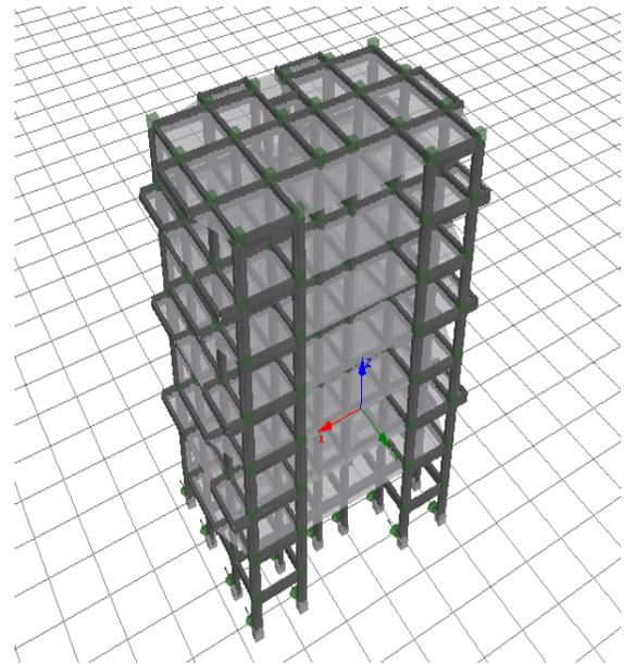
Fig 3: SeismoStruct model of G+7 Building
