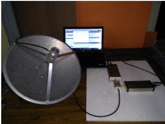
Fig -9: Experimental setup for return loss measurement of prototype.
