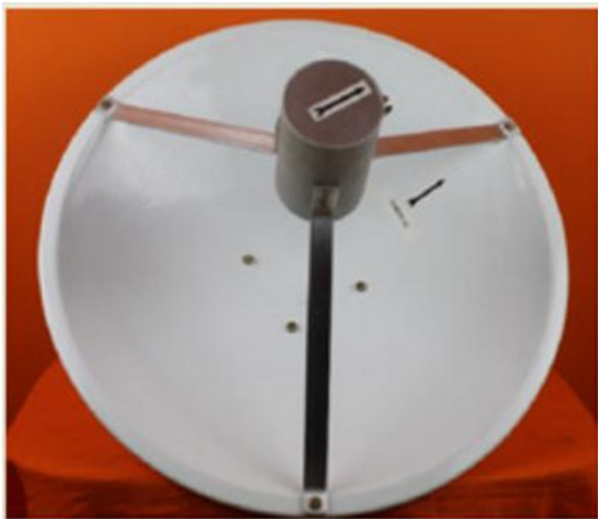
Fig -4: A front feed parabolic reflector antenna.
