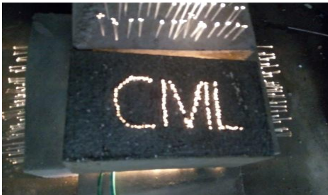
Fig.15: Light transmitting block under natural ventilation
