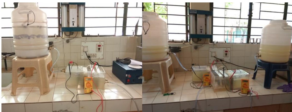
Fig 1: Experimental Setup of Dual Compartment – Microbial Fuel Cells.
