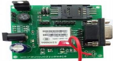
Figure 11: GSM Modem
