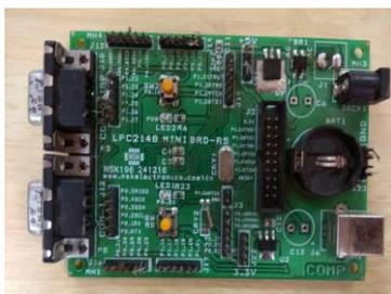
Figure 7: ARM7 Microcontroller Board
