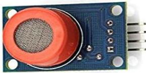
Figure 4: MQ3 Alcohol Sensor
