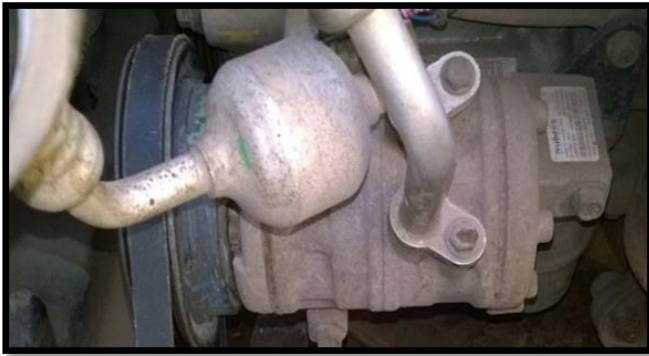
Fig -5: Swash Plate Type Compressor
