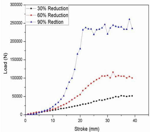
Load vs. Stroke with 30%, 60% & 90% Reduction (FEA)
