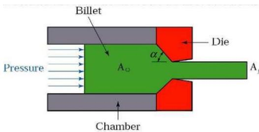
**1.2 The classification of extrusion processes are as follows,**
