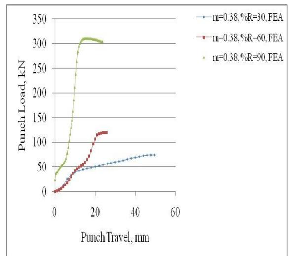
Load vs. Stroke with 30%, 60% & 90% Reduction (FEA)
