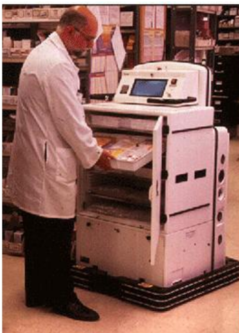
Fig.1. Drugs loaded in the Helpmate by a hospital pharmacist for delivery to staff in a hospital ward.
