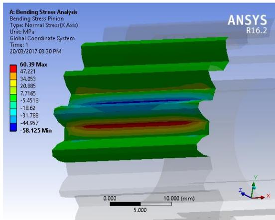
Fig-C: Bending stress in involute pinion
