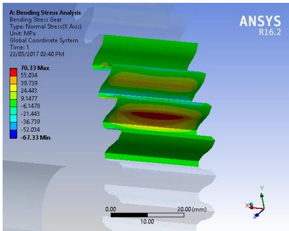
Fig-B: Bending stress in cycloidal gear
