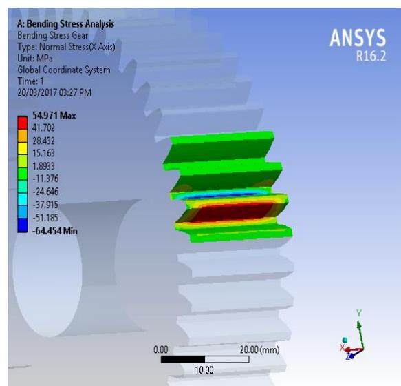
Fig-A: Bending stress in involute gear
