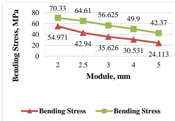
**Chart-2:** Variation of bending stress with different modules for involute and cycloidal gear teeth
