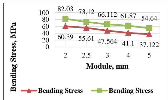
Chart-1: Variation of bending stress with different modules for involute and cycloidal pinion teeth
