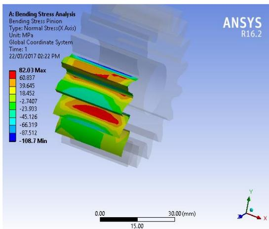
Fig-D: Bending stress in cycloidal pinion
