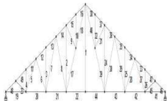
Fig-1: Model showing the beam numbers of truss
