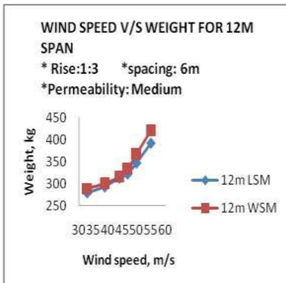
**Graph -1:** Showing the weight in Kg for 12 m span under different wind speeds in LSM and WSM for medium permeability
