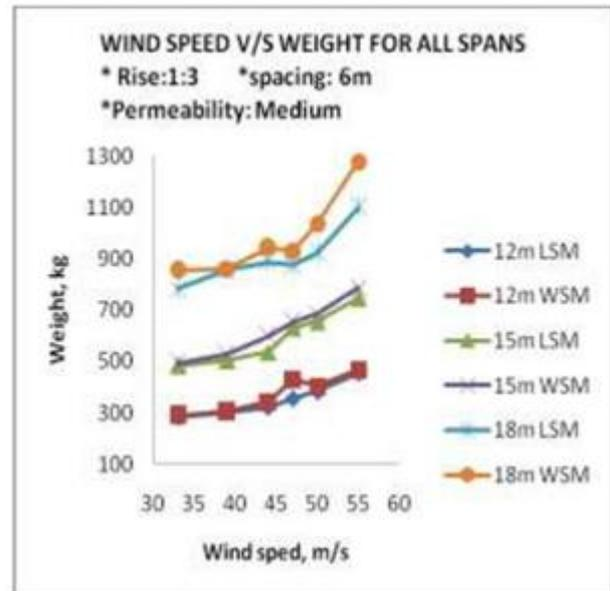
**Graph -2:** Showing the weight in Kg for 12m, 15 m and 18m spans under different wind speeds in LSM and WSM for High permeability
