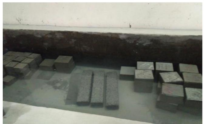
**Fig. 1.2.2Curing tank of cubes and prisms**
