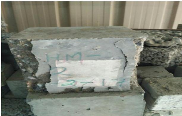
Fig.2.4 Cubes after compression testing
