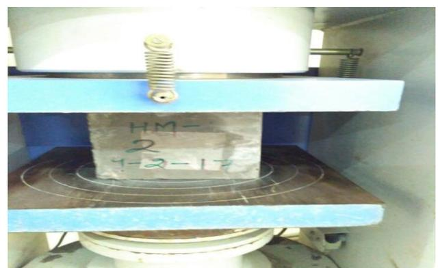
**Fig.2.3 Cube placed in testing appartus**
