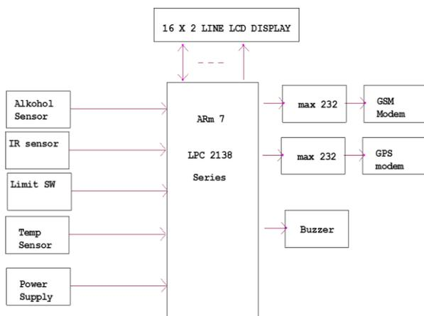
Fig. Block Diagram of Smart Helmet
