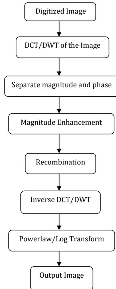
Fig.1 Block Diagram of Proposed Technique
