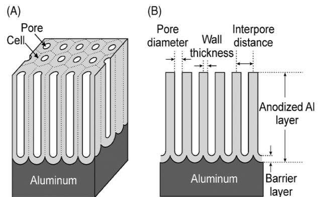
**Fig - 2:** Idealized structure of anodic porous alumina (A) and a cross-sectional view of the anodized layer (B). [3]
