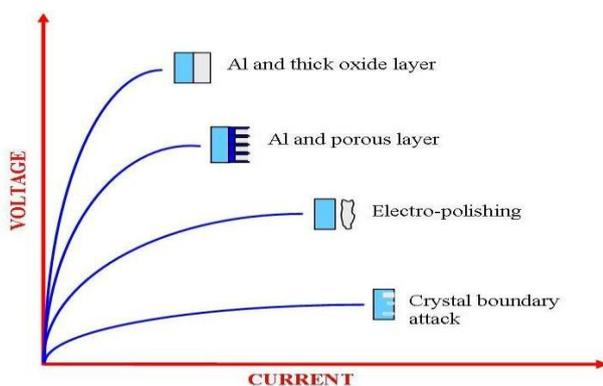
**Fig- 1:** Occurrences of changes on an Al. sample; represented on voltage vs. current plot [1]
