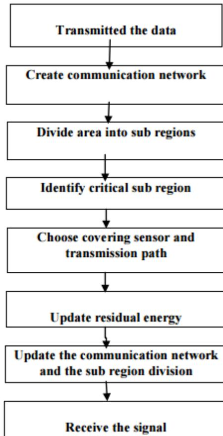
Fig-2 Data Transmitter and Receiver structure
