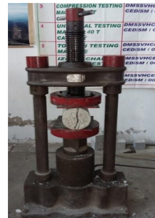
Fig – 7: Split Tensile Test
