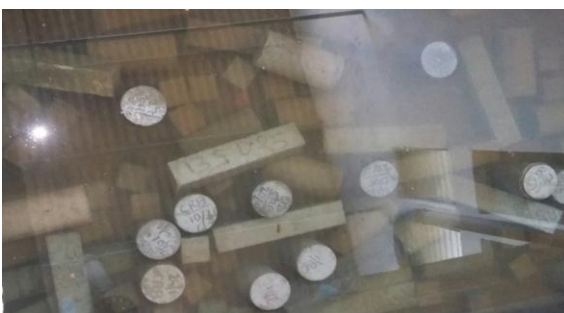
Fig – 5: Curing of specimens
