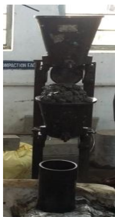
Fig - 2: Compaction factor test
