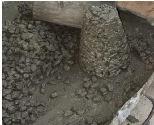
Fig - 1: Slump cone Test
