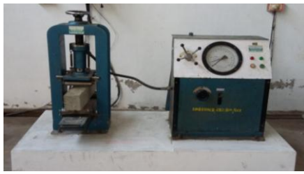
Fig - 8 : Flexural strength Tesing Machine
