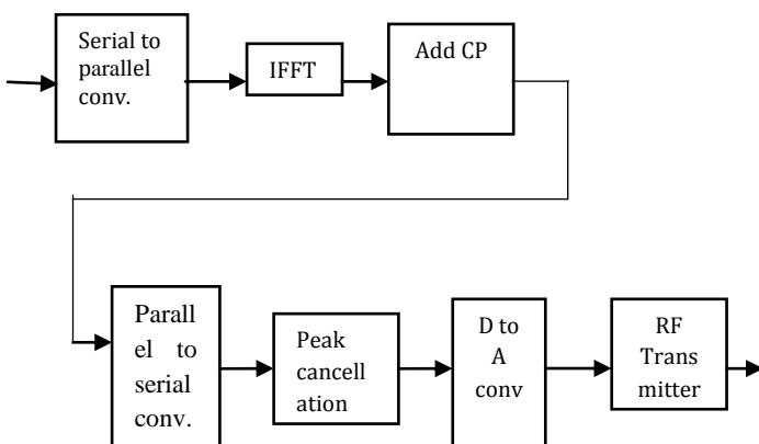
Fig.1: Basic block diagram of Peak cancellation
