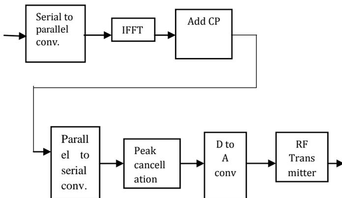
Fig.1: Basic block diagram of Peak cancellation
