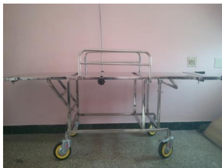
Fig. 3.3: Overall view of stretcher position with ss sheets
