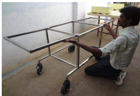
Fig. 3.2: Assembled view of outer frame and base
