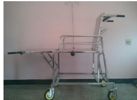
Fig. 3.4: Top plate foldable with SS sheets
