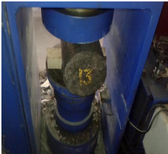
Fig -3: set up for split tensile test.
