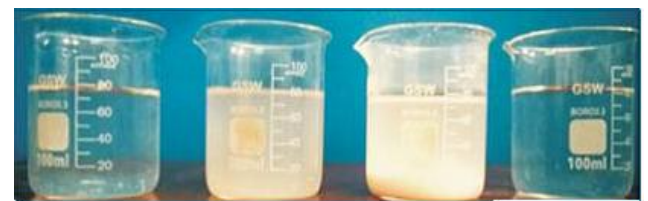
Fig -3.3: Preparation of MgO/water nanofluid.
