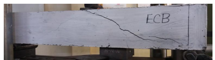
Fig -7: Failure pattern of control beam
