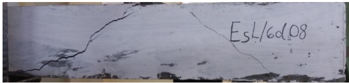
Fig -8: Failure pattern of EsL/6d08
