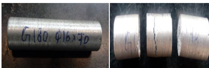
Fig: 12 Specimen before testing [Ø16mm] and after testing
