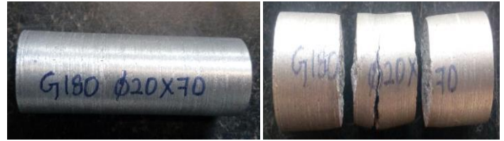
Fig: 13 Specimen before testing [Ø20mm] and after testing
