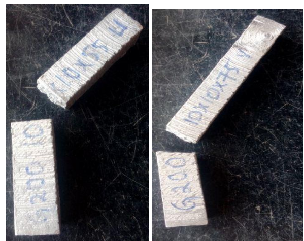
Fig: 10 Charpy and Izod Specimen after Testing
