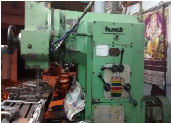
Machine used for Friction Stir Welding
