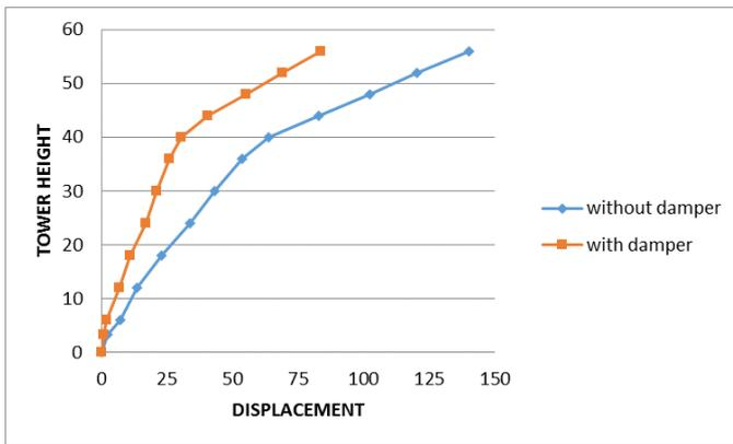
**Chart-2:** Graph showing Comparative values for tower height versus displacement
