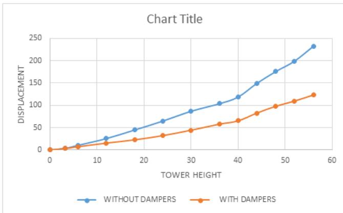
**Chart-1:** Graph showing Comparative values for tower height versus displacement
