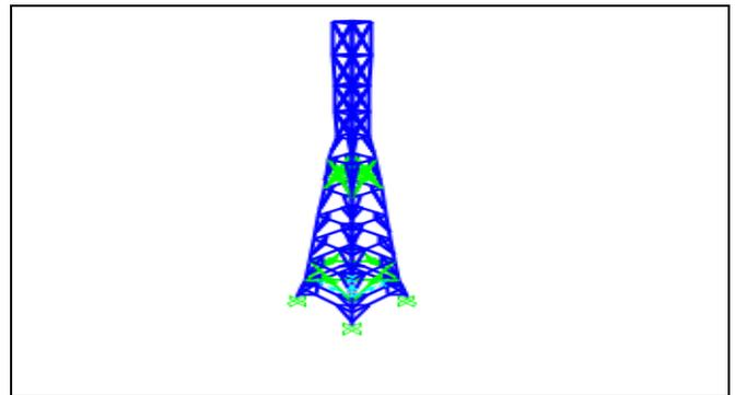
Fig 6: Telecommunication tower with dampers
