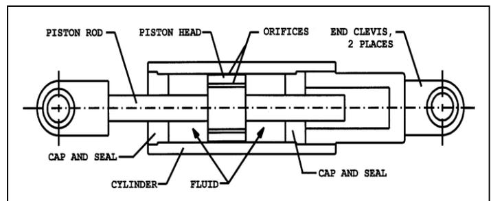
Fig 2: Fluid viscous Damper
